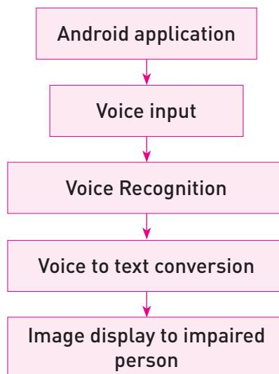
**Fig 2 : Flow diagram for voice to image conversion**
