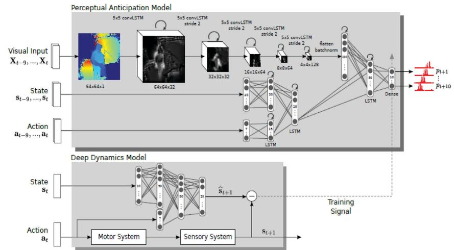
Fig. 1 : Architecture of Deep Predictive Model for perturbations [3].
