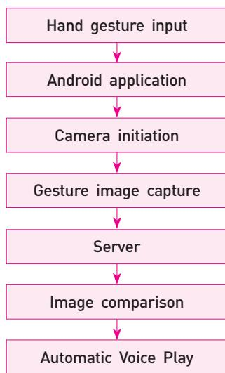
**Fig. 3 : Flow diagram for gesture to voice conversion**
