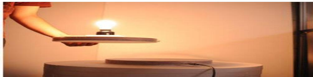
from a flat coil in the charger to a similar one in the device.
